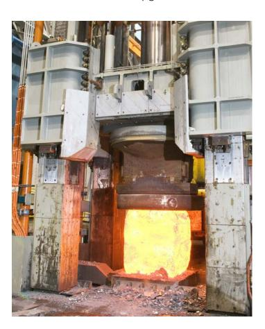
forging equipment components. The superior hardenability of ExELL™ 4330Mod enables excellent through hardness characteristics in section sizes greater than 25" in thickness.
